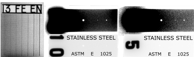
Figure 1. Left: X-ray image of a wire penetrator 13 FE EN (EN 462-1) on 6 mm steel. The smallest visible wire has a diameter of 0.05 mm. Middle and right: X-ray images of ASTM-E-1025 penetrators. Both measured on 6 mm steel. Middle: Thickness: 0.1" = 1T-hole. Right: Thickness: 0.05" = 1T-hole. The 1T-holes are clearly visible
