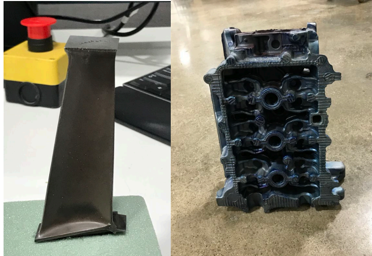
Figure 5: Objects scanned for the CBCT reconstructions at 450kV. Inconel turbine blade (left) and aluminum motorcycle cylinder head (right).
